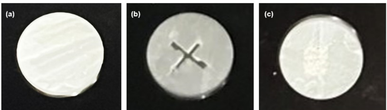
Figure 3: Silicone samples: (a) Control sample, (b) Sample with cross-shaped cut, (c) Sample with sponge. The images were taken while each sample was loaded in the sample holder, the visible portion of each sample has a diameter of 10 mm.
